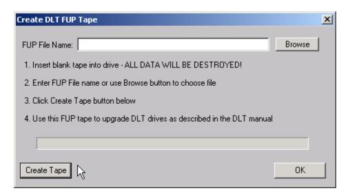
This command allows you to create an update tape from a firmware file. Use the Browse button to specify the firmware file name, then click the Create Tape button. You can then use this update tape to upgrade the firmware in other DLT tape drives.
